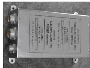
Fig. 14. Expected view of the Liulin-L particle telescope
