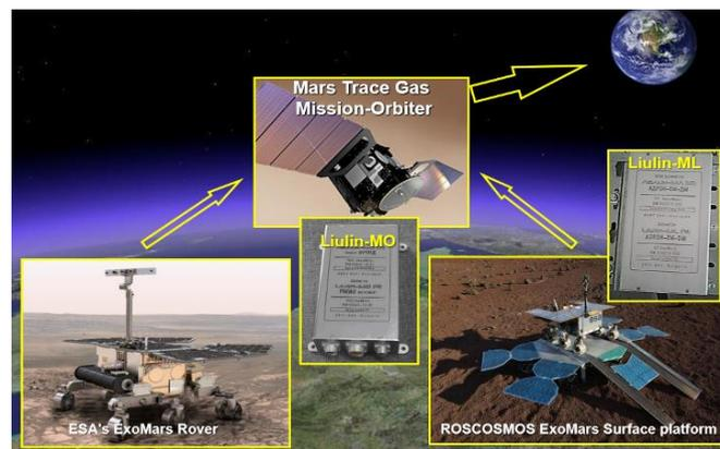
Fig. 7. Schematic presentation of the experiments with the Liulin-MO and Liulin-ML instruments on ExoMars TGO around Mars and in the surface platform at Mars
