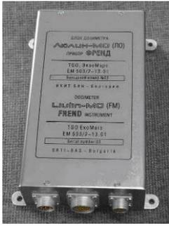
Fig. 1. Liulin-MO particle telescope
